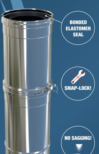
PowerStack EPSC is a single wall stainless steel venting system designed with the commercial installer in mind. A factory-installed integral seal and "no-tool" snap-lock assembly, makes it a go-to product for any commercial condensing applications offering reduced installation time for the installer.
