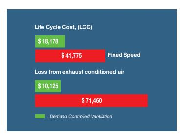
Fig. 14: Lifecycle cost of demand controlled versus constant speed ventilation systems
